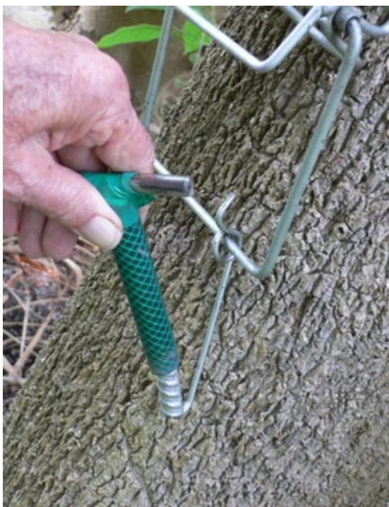
If you need to adjust curve in trigger drill a 4.5 mm hole 20 mm deep in the end of a piece of steel. Don't use pliers they mark the wire
