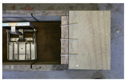
Drill 3x 4mm holes through top plate of box only, Don't drill into the extension. Angle the hole closest to the trap. Fix in place with 3x 8g 65 mm screws. Refit the inner mesh, making sure that the opening is on the treadle side.
